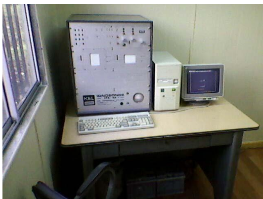
Photo 2: Ionospheric Prediction Service ionosonde IPS-42.
