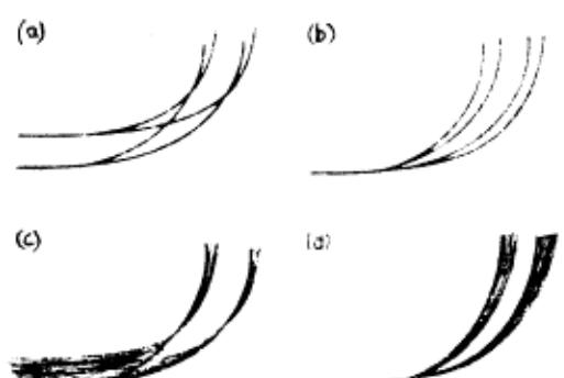
Figure 1. Ionogram sketches of (a) resolved range-spreading; (b) resolved frequency-spreading; (c) unresolved range-spreading; (d) unresolved frequency-spreading.
