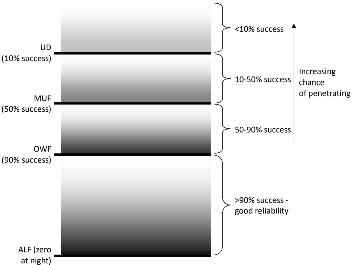
**Figure 1.** Upper and lower frequency limits for HF sky wave communications.
