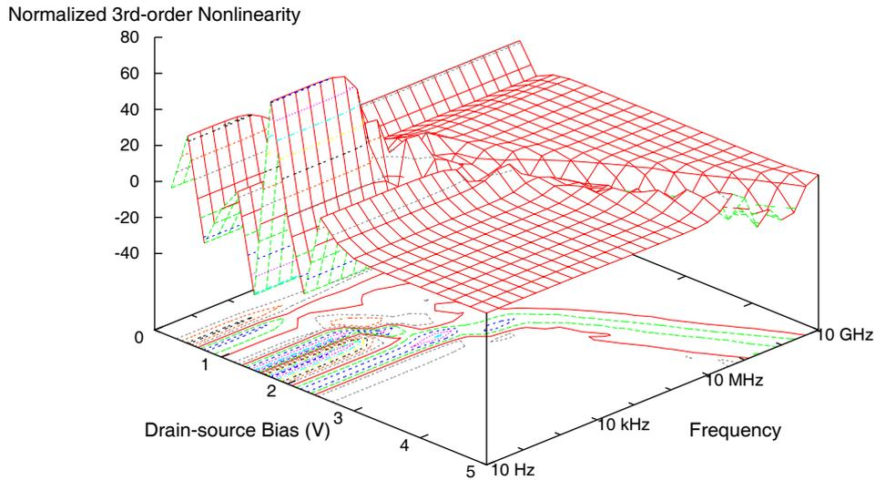
Fig. 7. A simulation at a  $-0.8\text{V}$  gate bias of the third-harmonic output for normalized to that at 10 GHz for a drain bias of 3 V. This shows the third-order nonlinearity relative to that of the isodynamic characteristic.
