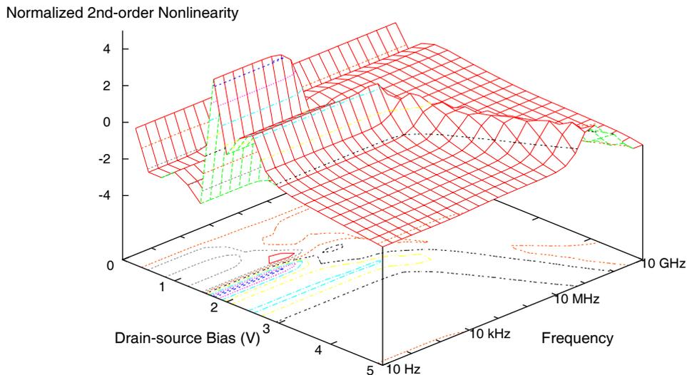
Fig. 8. A simulation at a  $-0.8\text{V}$  gate bias of the second-harmonic output normalized to that at 10 GHz for a drain bias of 3 V. This shows the second-order nonlinearity relative to that of the isodynamic characteristic.
