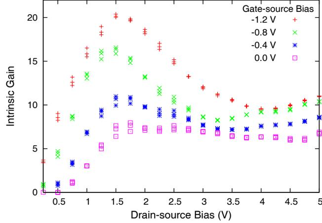
Fig. 4. Magnitude of *static* intrinsic gain of the same pHEMT in Fig. 1. This is the data at 10, 20 and 50 Hz for four gate-source potentials (one of which is that of Fig. 1). These are considered approximately *static* because the test frequencies are so low.
