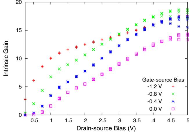
Fig. 2. Magnitude of *isodynamic* intrinsic gain of the same pHEMT in Fig. 1. This is the data at 1, 3, 5 and 10 GHz for four gate-source potentials (one of which is that of Fig. 1). These are considered *isodynamic* because they are constant with respect to increasing frequency.
