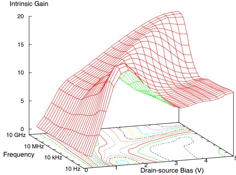
Fig. 1. Magnitude of intrinsic gain of a pHEMT biased at a gate-source potential of  $-0.8$  V (about  $50\%$   $I_{DSS}$ ). This device is  $160\ \mu\text{m}$  wide and has a breakdown at  $V_{GD} < -10$  V. This surface exhibits the salient features of shape and magnitude that those at other gate-source biases exhibit, included those near pinch-off.
