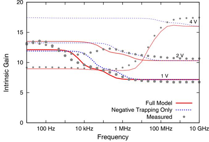
Fig. 5. Measured and modelled intrinsic gain for selected drain-source biases (as indicated) at a gate-source bias of  $-0.8$  V. The smaller points and thinner lines are for higher drain bias. Note that heating is not a significant effect for this device at these biases.
