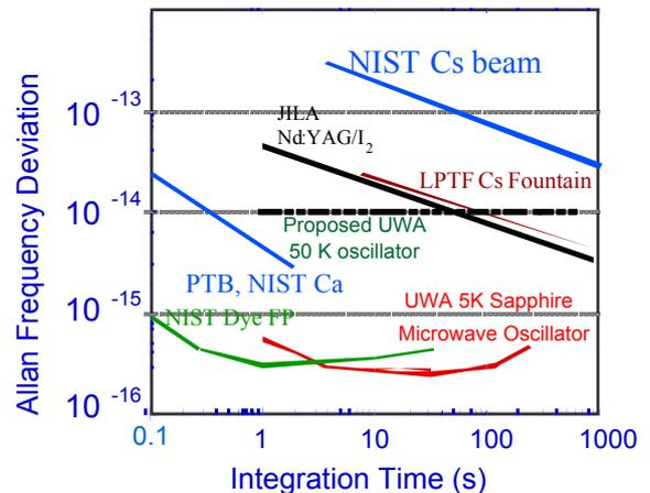
Fig. 2. State of the art frequency standards: Comparison of UWA microwave frequency standards with others worldwide. The UWA sapphire microwave oscillator has the best frequency stability over 3 to 1000 seconds.
