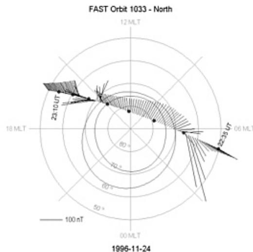
Fig. 2. Residual magnetic fields with the model IGRF removed on a FAST pass over the northern polar cap. The antisunward residuals near  $65^\circ$  are the signatures of region 1 and region 2 currents.
