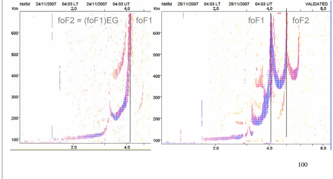
The correct scaling for foF2 is shown in both cases: when foF2 is not visible (the G condition) and when it is visible.
